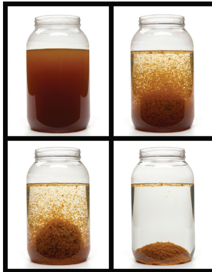
This series of photos shows what happens when a powdered purifier (Pur) is added to a polluted jar of water, killing bacteria and settling other pollutants such as floc.
