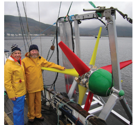
A contra-rotating marine turbine is ready to be installed.
